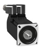
servo motor BMH, Lexium 32, 2.5Nm, 8000rpm, keyed shaft, without brake, IP54, 16bit encoder, 3 phases
