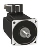
servo motor BMH, Lexium 32, 3.3Nm, 6000rpm, untapped shaft, without brake, IP54, 16bit encoder
