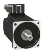
servo motor BMH, Lexium 32, 3.3Nm, 6000rpm, keyed shaft, without brake, IP54, 16bit encoder
