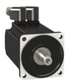
servo motor BMH, Lexium 32, 6.2Nm, 6000rpm, keyed shaft, without brake, IP65, IP67, 16bit encoder
