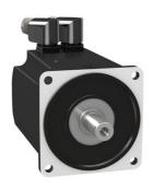
servo motor BMH, Lexium 32, 24Nm, 4000rpm, untapped shaft, with brake, IP54, 128 multiturn encoder, 3 phases
