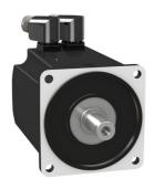
servo motor BMH, Lexium 32, 24Nm, 4000rpm, keyed shaft, without brake, IP54, 16bit encoder, 3 phases
