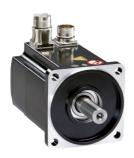
servo motor BMH, Lexium 32, 34.4Nm, 3800rpm, keyed shaft, with brake, IP65, IP67, 16bit encoder
