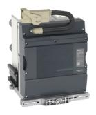
Disconnecting device, EasyPact EXE, basic function, 17.5kV, 31.5kA 3s, 2000A, 210mm, IEC
